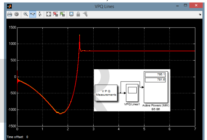
Figure.22. European Super Grid (HVAC) connecting Three European Countries with Three European Country Wind Farm generation drops to 800 MW (Case 04 Output Bus B5, B6)
