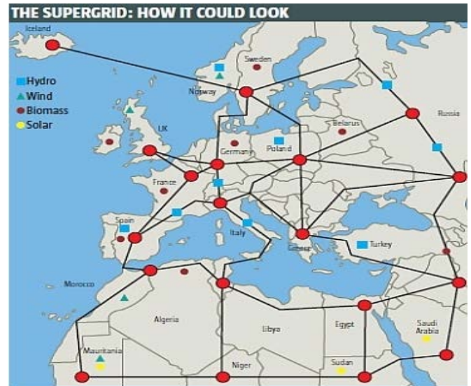
Figure.60. European super Grid (Interconnection of Wind, Solar, Biomass and Hydro Power Generation) [36]
