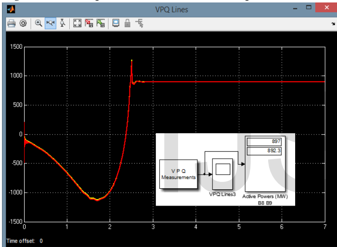
Figure.15. European Super Grid (HVAC) connecting Three European Countries with one European Country Wind Farm generation drops to 800 MW (Case 02 Output Bus B8, B9)
